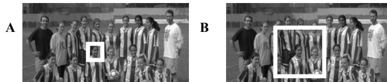
Figure 3: A local window (VJ) and a contextual window that captures relative position information from objects or parts around and within the detected object.
