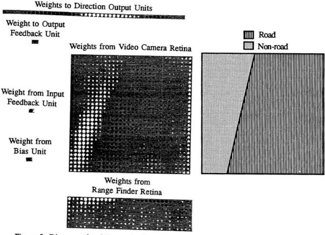
Figure 5: Diagram of weights projecting to and from a typical hidden unit in a network trained on roads with different widths.
