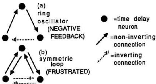
**Fig.5** (a) A ring oscillator: needs negative feedback at dc to oscillate. (b) Symmetrically connected triangle. This configuration is "frustrated" (defined in text), and has both oscillatory and fixed point attractors when neurons have delay.
