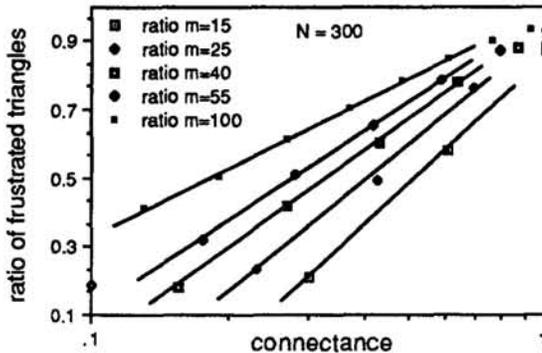
Fig.12 The number of frustrated triangles in a (+,0,-) Hebb rule matrix (300x300) divided by the expected number in a random signed graph with equal connectance. The different sets of points are for different numbers of random memories in the Hebb matrix. The lines are guides to the eye.
