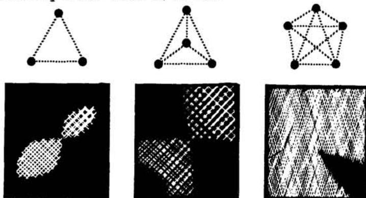
Fig.8 Size of basin for oscillatory mode increases with size of frustrated clique. The delay is  $0.46RC$  per neuron in each picture. Slices are in the space of initial voltages on neurons 1 and 2, other initial voltages near zero.
