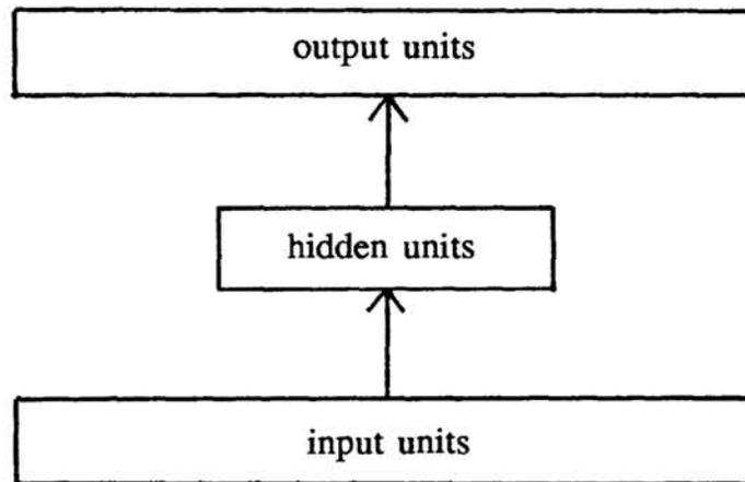
Fig. 1. A diagram of a three layer encoder network that learns good codes using back-propagation. On the forward pass, activity flows from the input units in the bottom layer to the output units in the top layer. On the backward pass, error-derivatives flow from the top layer to the bottom layer.
