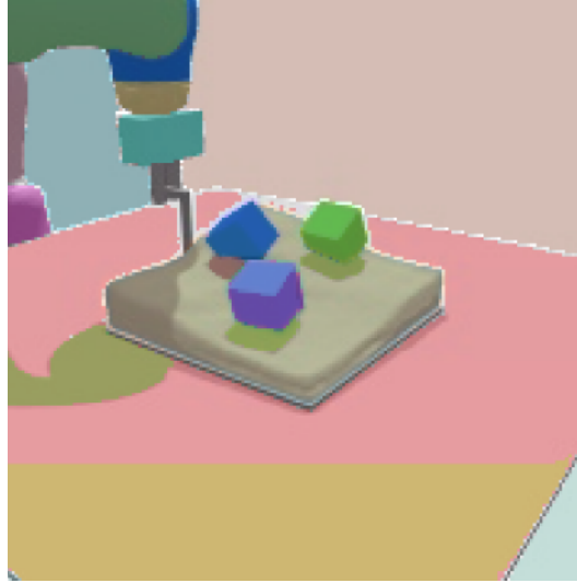
Figure 6: SAM Working on FluidCube Shake: Recent large segmentation models can well generate masks for different objects in the scene.
