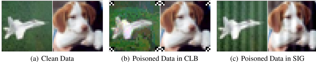
Figure 7: Examples of poisoned CIFAR-10 images at the training time ( Left ) and the test time ( Right ). Given the target label (class 0, “plane”), CLB and SIG instead attach a predefined trigger to some training samples belonging to target label to avoid incorrect labels at the training time.
